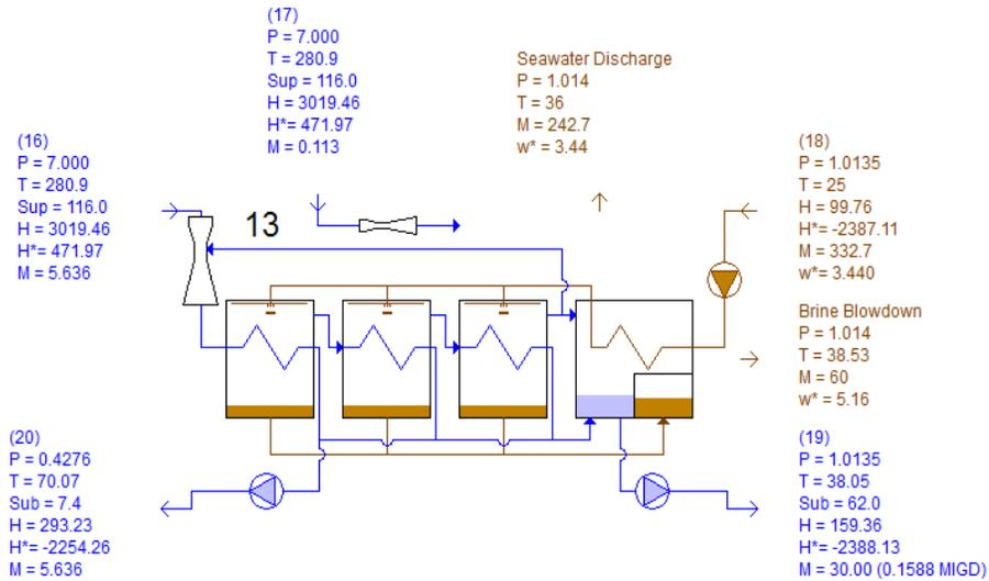
Fig. 5. MED plant, P[bar], T[C], H[kJ/kg], M[t/h]
