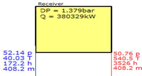
**Fig. 2.** Solar tower receiver, p[bar], T[C], h[kJ/kg] m[t/h]
