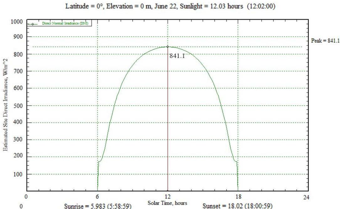
Fig. 3. Direct irradiance versus time
